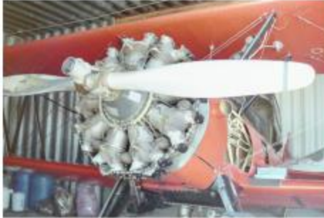
Metalized fuselage with Wright 475
