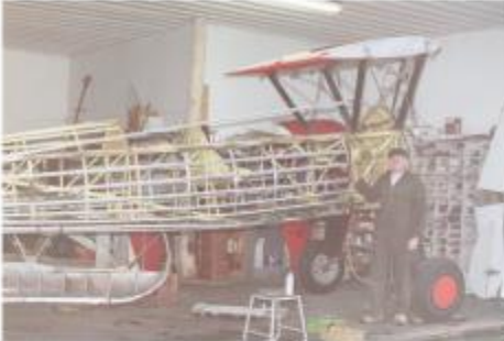
Fuselage with new "bird cage"
