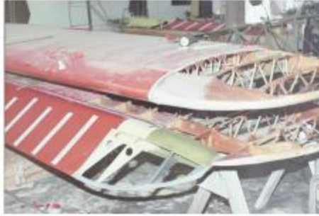
Restoration of ailerons and wing bows
