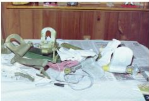
Restoration of rudder pedal system
